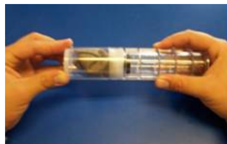
Step 5: Install cap, lips of part facing out, by pushing it evenly into cartridge and packing bean bag snugly.
