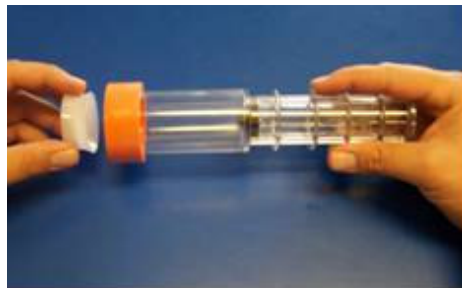
Step 2: Install the piston by pushing it into install tool
